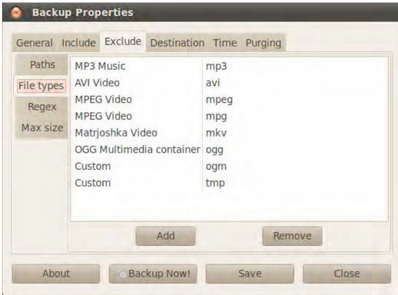
Figure 23-3. Excluding certain types of large files leads to far smaller backup files.
