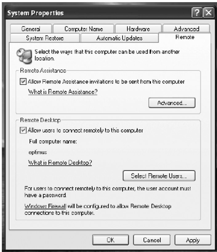
Figure 25-4. You need to enable the option under Remote Desktop to access Windows XP Professional machines using RDP and the Terminal Server Client program.
