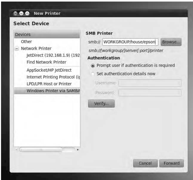
Figure 7-14. Ubuntu should be able to automatically detect any Windows or SMB shared printers on your network.
