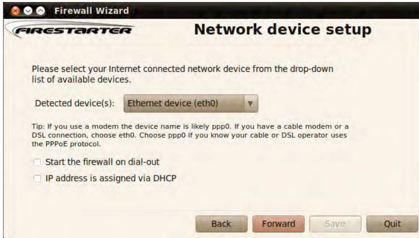
Figure 8-16. Firestarter includes a wizard to walk you through the basics of firewall configuration.
