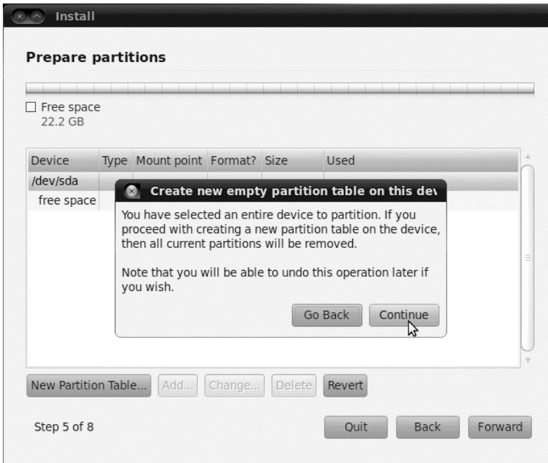
Figure 4-7. Creating a new partition table has the same effect as completely wiping the contents of a disk. Use with extreme care.
