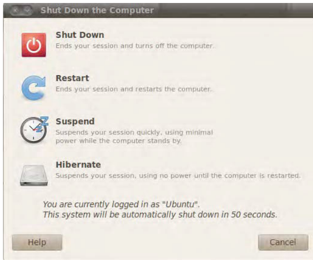
Figure 6-4. A variety of shutdown operations are available, some allowing for a quick resumption later on.
