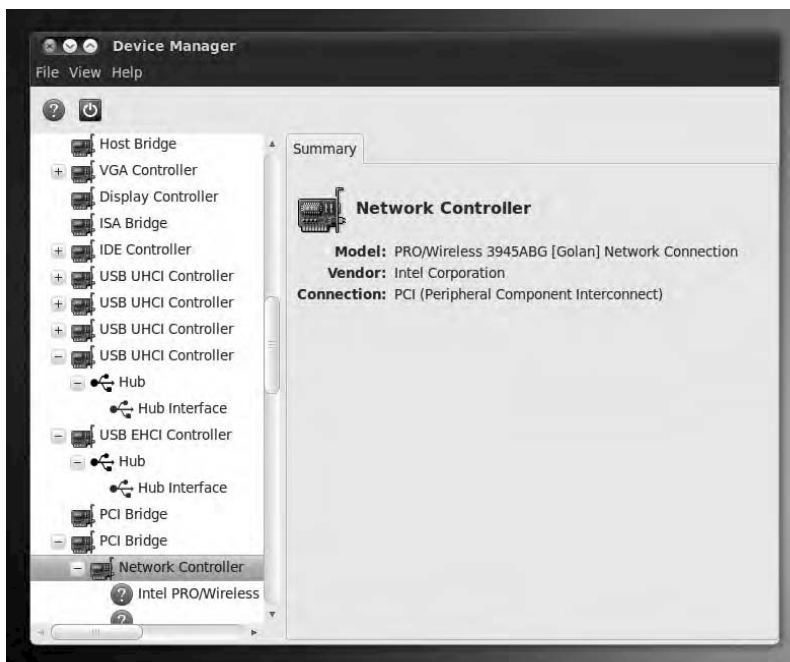
Figure 7-1. Ubuntu's Device Manager program can display just about everything you need to know about attached hardware.
