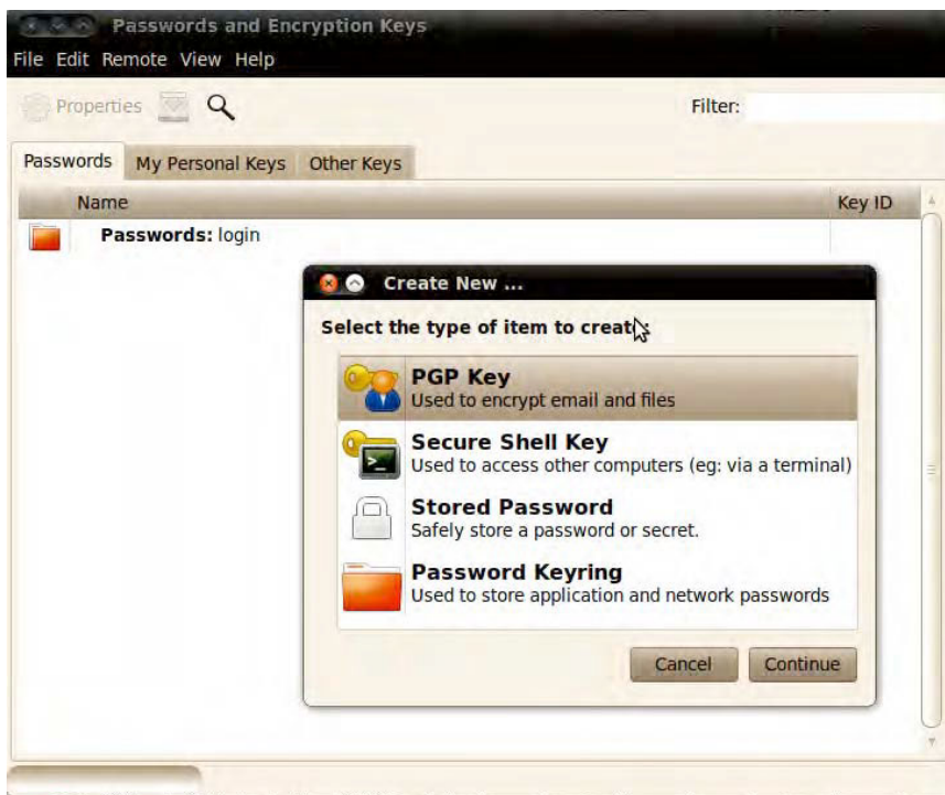
Figure 8-2. Choose PGP Key to create a key pair for e-mail or file encryption.
