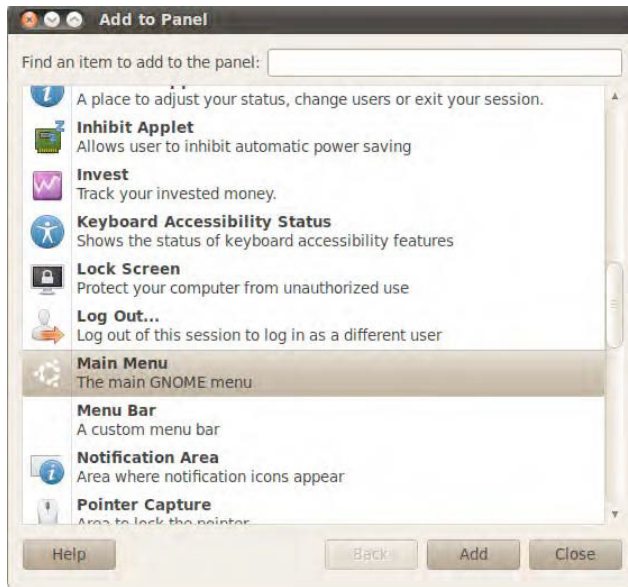
Figure 9-17. Use the Main Menu applet to add a Windows-like Start button to any panel on your screen.
