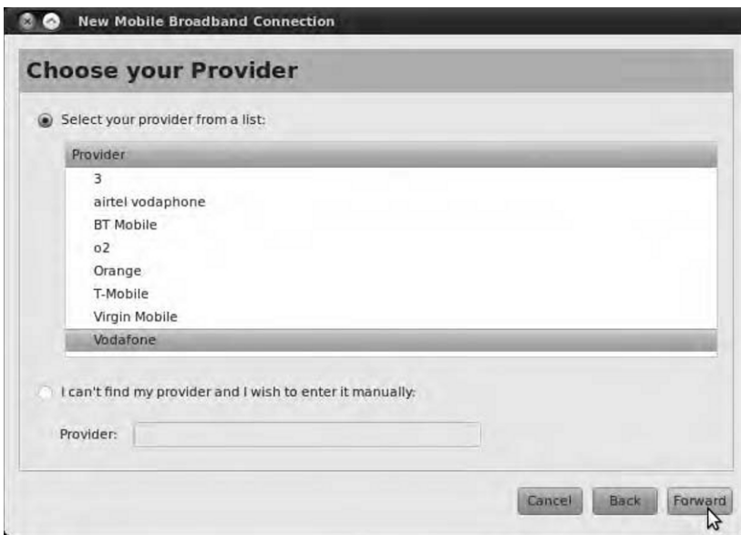
Figure 7-9. Ubuntu's mobile broadband connection wizard makes it straightforward to set up a 3G link.
