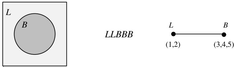
Figure 10.53: Optimal segmentation and interpretation: interpretation, corresponding code string, and region adjacency graph. © Cengage Learning 2015.
