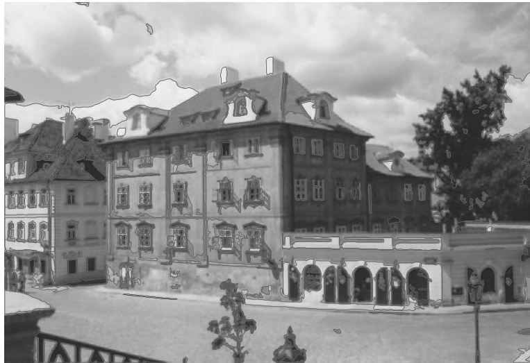
Figure 5.35: MSERs: Red bordered regions are results of the algorithm on the increasingly ordered list of intensities. Green bordered regions come from the list with decreasing ordering. Courtesy of J. Matas, Czech Technical University, Prague. A color version of this figure may be seen in the color inset—Plate 8.
