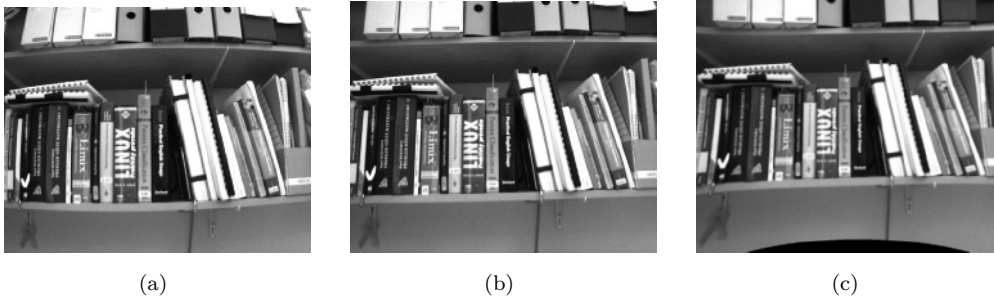
Figure 3.36: Radial distortion illustrated on an image of a book shelf. (a) Barrel distortion. (b) Undistorted. (c) Pincushion distortion. © Cengage Learning 2015.
