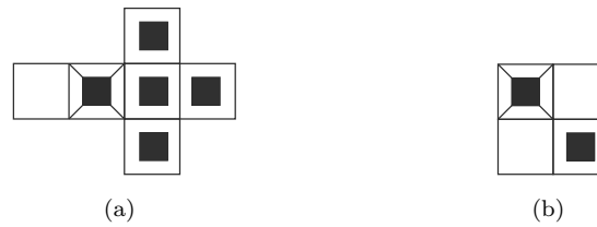
Figure 8.32: Masks for the MB skeletonization algorithm [Manzanera et al., 1999]. All 90-degree rotations of these two are included. Panel (a) shows the thinning mask (plus all \pi/2 rotations). Panel (b) shows the restoring mask (plus all \pi/2 rotations). The central mask pixel is marked with a diagonal cross, background pixels are white and object pixels are black. © Cengage Learning 2015.
