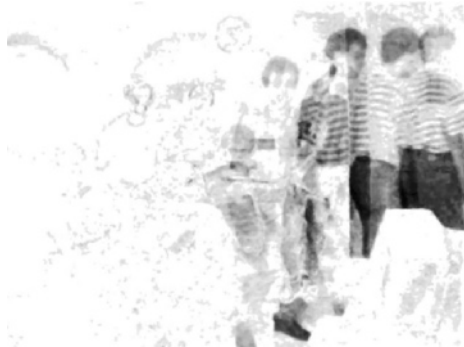
Figure 16.3: Cumulative difference image determined from a sequence of five frames depicting motion analyzed in Figure 16.2 (inverted for improved visualization). © Cengage Learning 2015.
