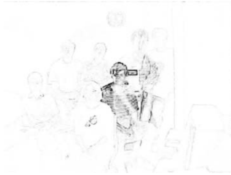
Figure 16.5: Moving-edge image determined from the first and second frames of the image sequence analyzed in Figure 16.2 (inverted for improved visualization). © Cengage Learning 2015.
