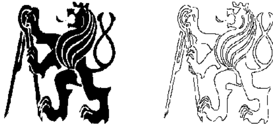
Figure 13.9: Contours obtained by subtraction of an eroded image from an original (left). © Cengage Learning 2015.
