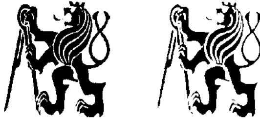
Figure 13.8: Erosion as isotropic shrink. © Cengage Learning 2015.
