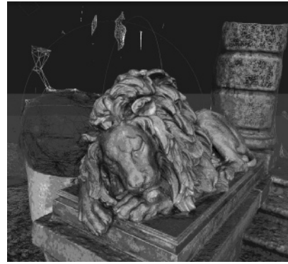
Figure 12.31: The same view with a triangular mesh built on top of the point cloud from Figure 12.30. Courtesy of T. Pajdla, M. Jancosek, C. Albl, Czech Technical University in Prague.
