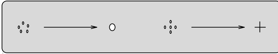
Figure 15.16: Primitive grouping—low-level primitive patterns are grouped into single primitives at a higher level. © Cengage Learning 2015.
