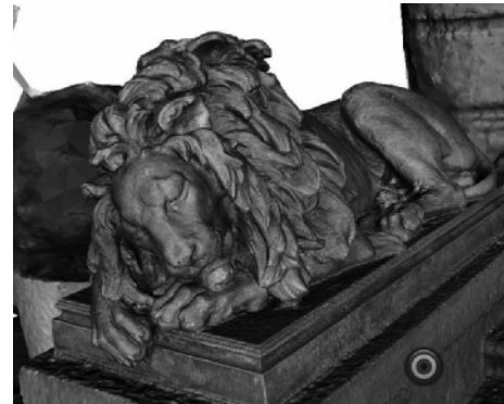
Figure 12.33: The same view where the triangular mesh is colored (gray level here) by the appropriate color from input images. Courtesy of T. Pajdla, M. Jancosek, C. Albl, Czech Technical University in Prague.
