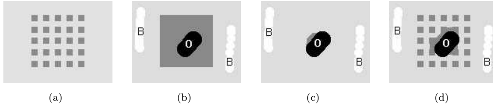
Figure 7.37: Graph cut segmentation behavior on a synthetic image. In all cases, the segmentation was initialized using the object patch as marked in black and background patch marked in white. The resulting segmentation is shown in light gray (background) and dark gray (objects). The initialization patches are parts of the segmented object(s) or background. (a) Original image. (b) Segmentation result for \lambda \in [7, 43] , i.e., only using a wide weighting range of region and boundary cost terms. (c) Segmentation result for \lambda = 0 , i.e., only using the boundary cost term. (d) Segmentation result for \lambda = 60 , i.e., using almost solely the region cost term. Notice the ability of the method to change the topology of the segmentation result. Courtesy of Y. Boykov, University of Western Ontario. © 2001 IEEE. Reprinted, with permission, from Y. Boykov and M.-P. Jolly, “Interactive Graph Cuts for Optimal Boundary & Region Segmentation of Objects in N -D images,” International Conference on Computer Vision, (ICCV) , vol. 1, pp. 105-112, 2001.
