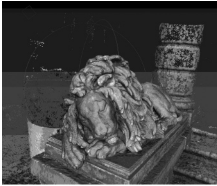
Figure 12.30: One view on the 3D point cloud. Each point is displayed in the color (here gray level) provided by input images. Courtesy of T. Pajdla, M. Jancosek, C. Albl, Czech Technical University in Prague.
