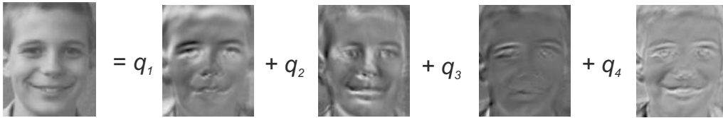
Figure 3.24: Reconstruction of the image from four basis vectors \mathbf{b}_i , i = 1, \dots, 4 which can be displayed as images. The linear combination was computed as q_1 \mathbf{b}_1 + q_2 \mathbf{b}_2 + q_3 \mathbf{b}_3 + q_4 \mathbf{b}_4 = 0.078 \mathbf{b}_1 + 0.062 \mathbf{b}_2 - 0.182 \mathbf{b}_3 + 0.179 \mathbf{b}_4 . © Cengage Learning 2015.
