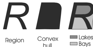
Figure 2.15: Description using topological components: An ‘R’ object, its convex hull, and the associated lakes and bays. © Cengage Learning 2015.
