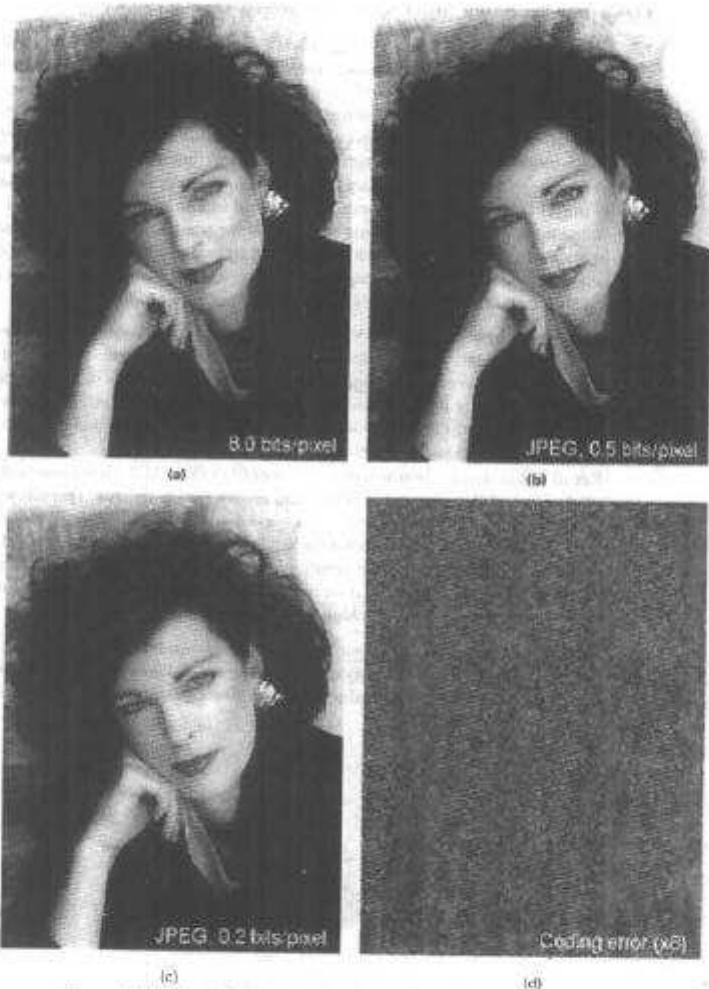
Figure 17-4 Examples of image compression: (a) original 560-by-764 pixel, eight-bit image; (b) JPEG compression at 0.5 bit per pixel; (c) JPEG compression at 0.2 bit per pixel; (d) difference image between (a) and (c), contrast times eight
